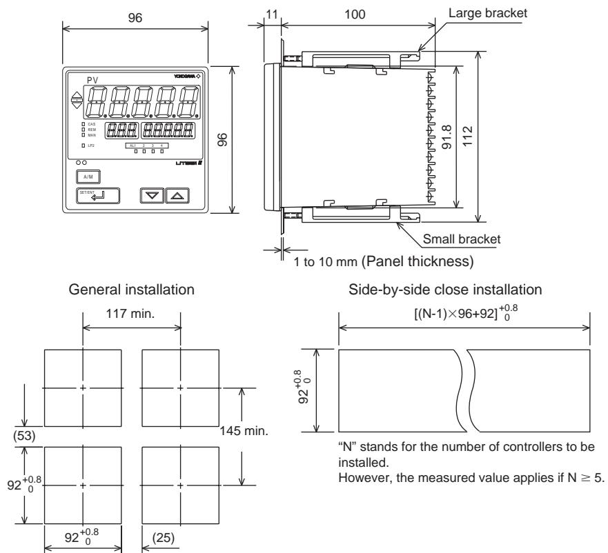
Normal Allowable Deviation=± (Value of JIS B 0401-1999 tolerance grade IT18) /2
